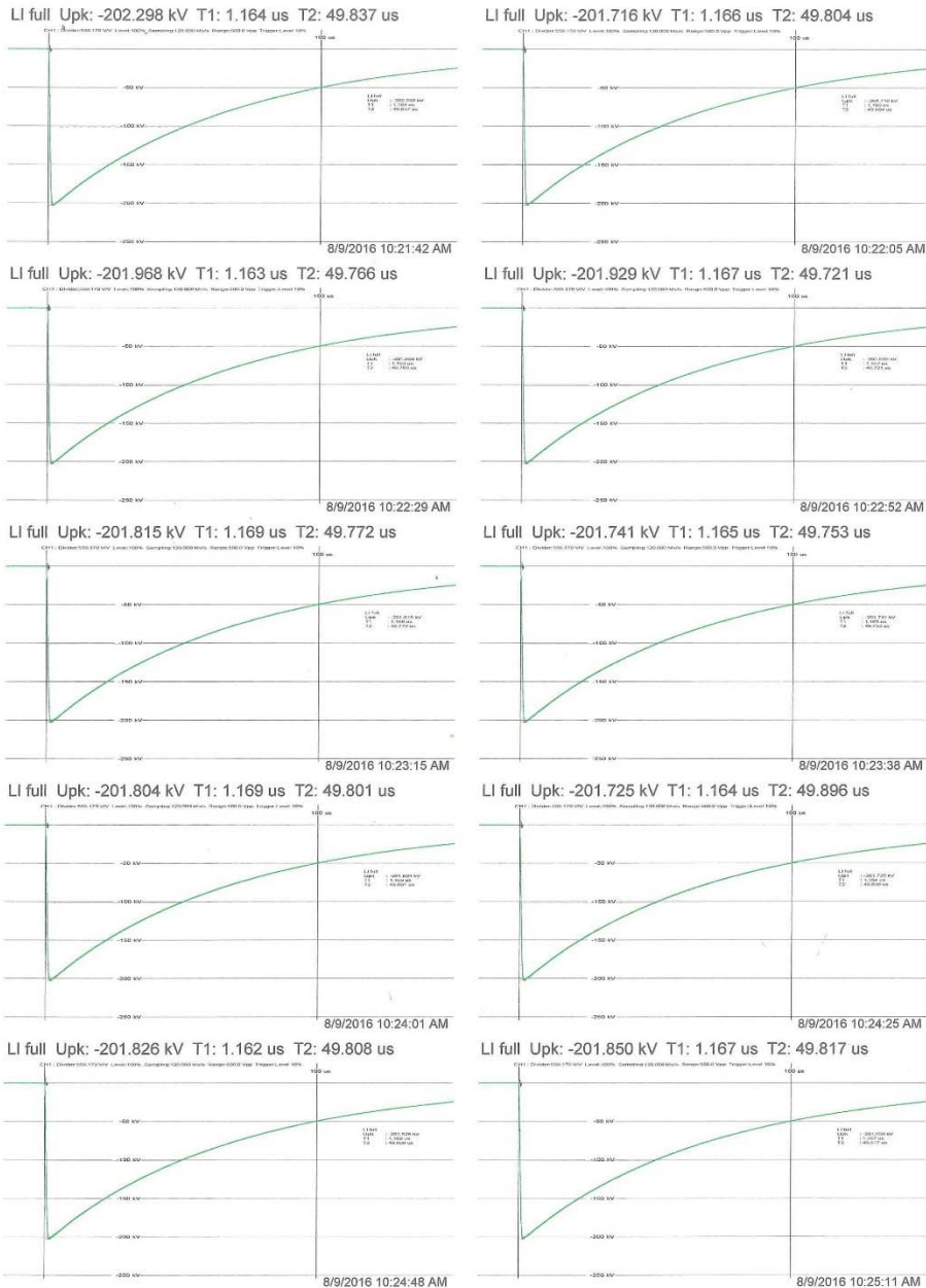
Fig. 1: Impulse oscillograms for 185mm 2 XLPE cable, loop 1- 4
